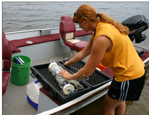
Lake monitoring equipment. The water sampler collects water to be tested for nitrates, phosphorus, calcium, aluminum, and chlorophyll a.
